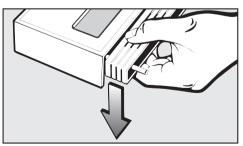
To remove the spacer bars from the control panel, place the panel on a table, printed side up, and gently push down on the spacer bars at a point near the bottom of the control panel. This will release the mounting bolts from their slots.
